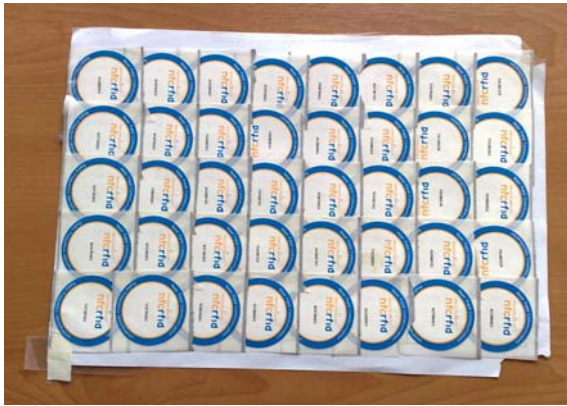
Figure 7. Modular tile with 40 overlapping NFC-tags
